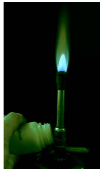
Anhydrous salt aspirated into air jet of Bunsen burner.
