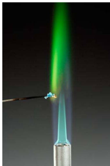
Wire or wood splint with small amount of solid chemical.
